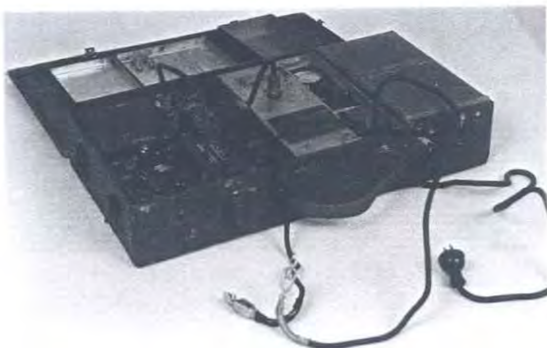
The SSTR-1 wireless telegraphy, short-wave radio transmitter and receiver in its suitcase carrying case complete with battery on the right and wires for connection to the battery and a plug for use with an electrical outlet. The battery was recharged by hand crank. Courtesy of John W. Brunner.
